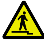
下り段差注意 Caution, uneven access/down
