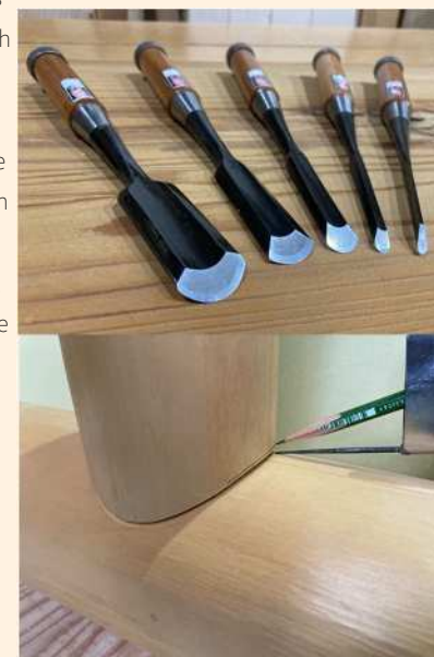
Round chisel actually used by craftsmen (upper) Tough work of "hikarizuke" (lower)
